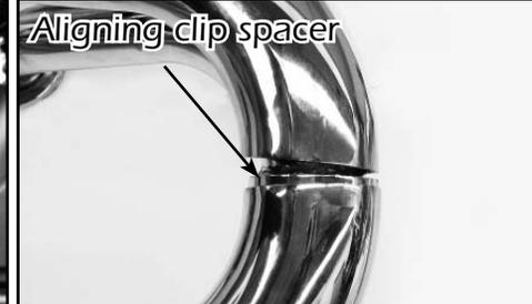
Aligning clip spacer
