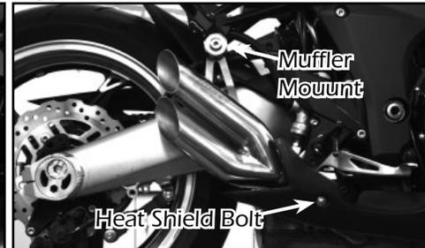
1. Starting on the right side, slide the muffler inlet into the collector outlet, using care not to damage the gasket.
