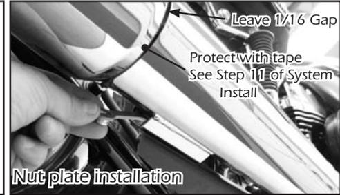
**Note: Black Ceramic exhaust systems require special care during installation. Applying low tack tape (painters or equivalent) to edges or areas where movement or scratching can occur during installation can be very helpful.**
