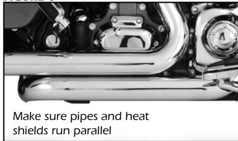
Make sure pipes and heat shields run parallel
