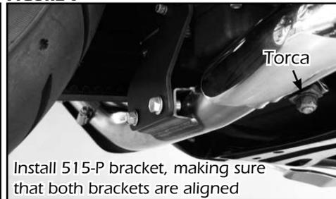
Install 515-P bracket, making sure that both brackets are aligned
