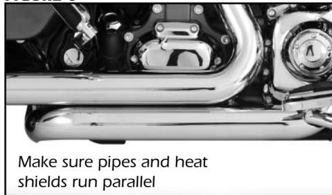
Make sure pipes and heat shields run parallel
