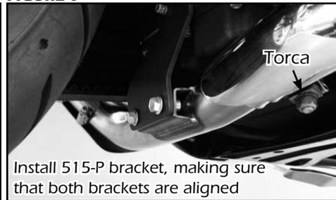
Install 515-P bracket, making sure that both brackets are aligned
